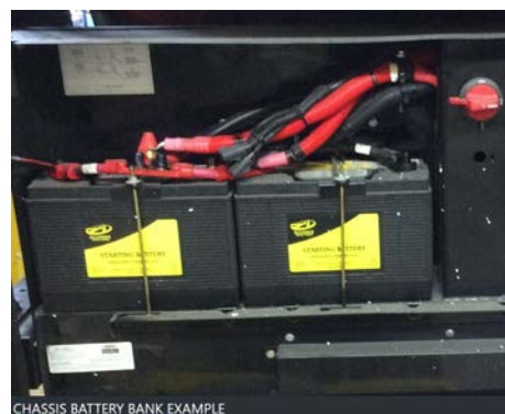
CHASSIS BATTERY BANK EXAMPLE
