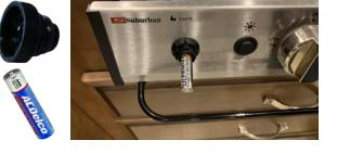
If the burners fail to light due to no spark, unscrew the ignitor cap. Check and replace the battery as needed.
