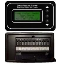
**Inverter/Converter Combinations:** Many Newmar coaches are equipped with inverter/charger combination units, sometimes referred to as inverter/converter units. These units range from 1200 to 3000 watts and serve as a three-stage charger and an inverter. Coaches equipped with this option will also be equipped with a 120 Volt subpanel.
