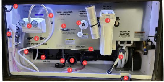
(1) Drain Outlet and Cover: The drain outlet is used to attach a 4" sewer hose, and the drain cover is used to prevent leakage of waste material. Make sure the drain cover is securely installed on the drain outlet unless actively dumping the tanks via a 4" sewer hose.
