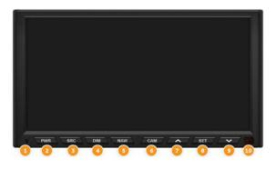
(3) AUX Zone: Allows you to select what output is displayed on the Passenger monitor. This is the same as using the SRC button that monitor.
