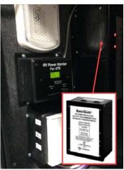
If there is no error message and the display instead reads "Delay Active" this means that the fault condition has cleared and that the switch is going through a 2.5 minute delay before it will attempt to close the contactor again. Wait until this delay is over to see if the ATS correctly closes its contactor.
