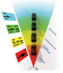
Adaptive Cruise Control (ACC) automatically adjusts the speed of your vehicle while in cruise control and attempts to maintain a set following an interval of 3.6 seconds when there is a vehicle ahead. ACC works with conventional cruise control to maintain the set cruise speed when the lane ahead is clear and will automatically adjust the vehicle's speed to maintain the set following interval when a vehicle ahead is detected.
