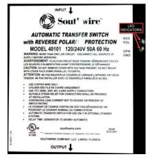
Reverse Polarity Indicator Illuminated: Unplug shore power. Use a voltmeter to check ground and neutral. Voltage should read -0-. If not, finding another power source is recommended.
