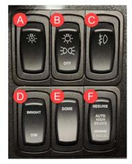
**(B) Headlamp Switch:** The headlamps can be turned on by the headlamp switch. In the first position, the switch will activate the marker, tail, identification, center, and clearance (ICC) lamps. The second position will activate the headlamps. While the headlamps are active, the turn signal lever can be pulled towards the driver to toggle between high and low beam operation. While vehicle ignition is on, an indicator in the instrument panel will be active whenever the high beam lamps are on.
