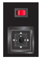
The red toggle switch located near the mirror adjustment control operates the mirror heat (if equipped). The ignition switch must be on for the mirror heat switch to operate.
