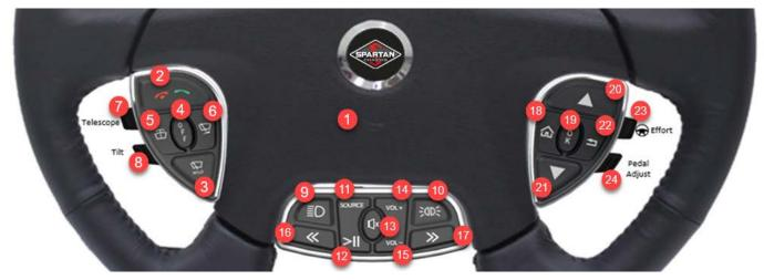
(1) Horn: The button for the horn is located in the center of the steering wheel. To sound the horn, press the center of the steering wheel pad.
