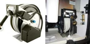
The hose reel deploys manually by pulling the hose outward from the compartment. Once the desired length of hose has been extended, hook up the hose to a potable water source. A switch located on the side of the hose reel requires activation for power retraction.
