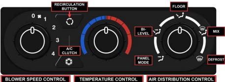
The Bergstrom vehicle A/C system will not function if the outside temperature is below approximately 40 degrees F. For cool air circulation during low temperatures, it is suggested the operator utilize fresh air mode.
