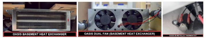
Set the thermostat zones on "Furnace" mode, and adjust each interior zone temperature setting as desired. The separate Oasis System must be turned on via the Oasis control panel, SilverLeaf touchscreen, or KIB touch panel (2024 and newer coaches), and the water temperature in the Oasis System must be up to temperature for the basement heat to work.
