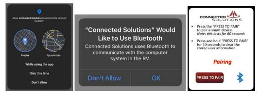
Enable paring mode by pressing the "PRESS TO PAIR" button on the ATCNET module (# 162818) with a paper clip or a pin or press the "PRESS TO PAIR" button on the ATCNET (# 158285) module. This enables pairing for 60 seconds.
