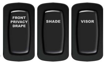
Press the UP or DOWN button for the appropriate shade. Switches may be labeled "Front Privacy Drape" or "Shade." Switch-operated shades require the switch to be held until the shade either reaches its limit or the desired intermediate position (the shade can be stopped at any point by simply releasing the switch).
