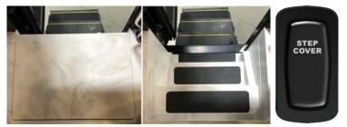
On select coaches, the switch for the interior step cover is located either on the side of the passenger console, on the dash console near the center, or near the mid-entry step well. Press the switch forward to extend the step cover to make it level with the coach floor. Press the switch backward to lower and retract the cover in the stored position.
