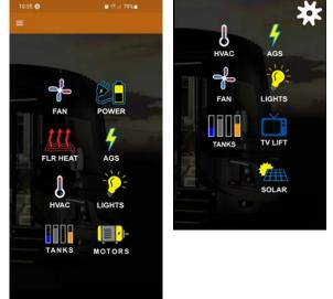
**MOTORS (TV LIFT):** Page jump to the TV LIFT page (must have factory-installed television lift option for this icon to appear).
