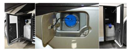
Some vehicles are equipped with a remote DEF fill-port. If so equipped, the remote port is directly opposite the DEF tank on the other side of the vehicle, and has a blue cap over the fill-port. DEF parts, such as the fill cap or tank, are supplied by the chassis manufacturer and are not available via the Newmar Parts Department.
