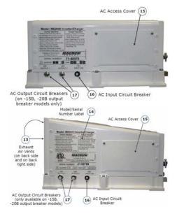
AC Output Circuit Breakers (CB1 & CB2): These circuit breakers are branch-rated and are only available on models MS2000-15B, MS2000-20B, MS2012-15B, MS2012- 20B, and MS4048-20B. They allow the inverter AC loads to be connected directly to the inverter's output without requiring an inverter sub-panel. These circuit breakers pop out when they open—press in to reset. They can also be manually pulled to disconnect the inverter's loads.
