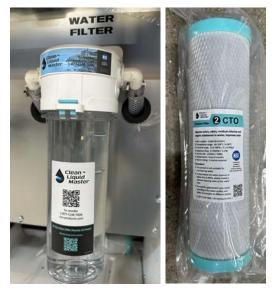
Change the filter at least every six months and at any time you notice decreased water flow or notice an unpleasant taste, odor, or algae after flushing and sanitizing the water system. Water filters and fresh water system maintenance are the customer's responsibility to ensure safe potable water.
