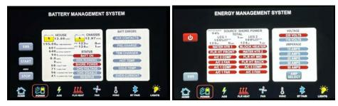
The Power button will allow the user to turn the Energy Management system on or off. When the EMS is off, it will allow the supply of power to all systems unregulated and may result in an overload of the incoming supply power and tripped shore power breaker(s).
