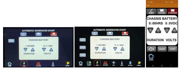
Example: If the house battery volts is "11.0 VDC" and the duration is "2:00 HRS," when the house battery voltage is less than 11.0VDC, there will be a demand for the generator to start and run for 2:00 HRS. The chassis battery works the same way but with its own settings.
