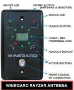
On coaches with a Rayzar automatic TV antenna, this switch is integrated into the power on/off switch typically located in the overhead control center.
