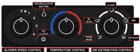
**Temperature Control:** The temperature control dial controls only the heat content of the discharge air. The temperature control dial will also control the overall temperature of the discharge air if the AC system is operating. Turn the knob to the right (red area) for warmer air, and to the left (blue area) for cooler air. Use of the temperature control will also moderate the discharge temperature when the cooling system is engaged.
