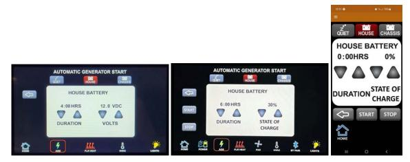
**Duration:** Time the AGS is to run the generator after a low battery demand occurs. Use "HR" & "MIN" buttons to set the amount of time the generator will run while charging the house or chassis batteries.
