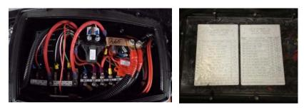
The fuse labels are attached to the cover and contain the fuse size. To reinstall the cover, place it over the panel, and rotate the retainer clips to hold it in place. Labels on the cover show fuse location, and amperage and have a general description of what the fuse powers.
