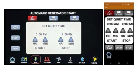
Note: The time of day is set in the HVAC section and must be set for operation. For example, RV parks have posted times when generators are not to run, and the user simply enters those times and enables the "QUIET" button on the status page. During this time, the generator will not run.
