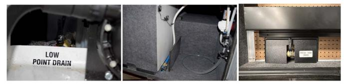
To drain the fresh water tank, open the low point drain valve located near the fresh water tank. The following images are example fresh water tank drain configurations. For more information, refer to the <u>How to Winterize a Coach</u> and <u>How to</u> <u>Sanitize the Water System</u> articles in Newgle.
