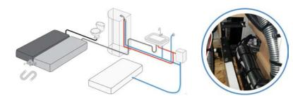
utilizing the coach water supply, are typically hard-plumbed within the slideout. To ensure flexibility, a braided hose connects the rigid plumbing from within the slideout to the rest of the plumbing in the coach. This hose easily moves with the slideout as it extends and retracts. The plumbing lines are normally tied to the flexible drain pipe and extend and retract smoothly as the slideout travels.
