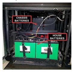
The chassis batteries are isolated from the coach batteries; however, when certain parameters are met, the BIRD, BIM, or charge bridge will activate and allow charge to the chassis battery. This prevents the chassis batteries from being drained by the interior 12 volt equipment, allowing ample voltage for engine ignition.
