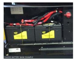
motorhome are installed by Newmar Corporation, but warranted by the battery manufacturer. These batteries are used to operate the 12 volt items that are not a direct part of the chassis.
