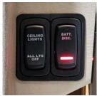
lights on the ATC/KIB network. The switch may be equipped with backlighting to provide better visibility in the dark.
