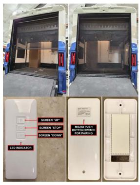
Source(s): Auto-Motion Shade Quick Reference Guide (QRG) # 9: Pairing of 2nd Generation RF Transmitters with Standard Motor 4280P, Using External RF Receiver Module 216P
