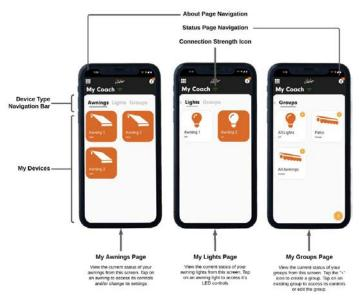
The light icon will indicate the status of your awning lights. An orange icon represents ON status and a white icon represents OFF status. Pressing the icon allows you to access the controls for the awning lights including ON/OFF, brightness, and color selection (if your RV configuration includes RGB LEDs)
