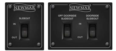
**Electric Bedroom Slideouts:** The operating switch for the bedroom slideout is usually located on the bedroom wall. If there is a full wall slideout on the driver side of the coach, the switch may be located on the wall that separates the bedroom from the living room.
