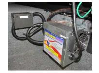
stage, the inverter charges at nearly its full current ability. This causes the battery voltage to rise over time. After the battery voltage reaches the bulk voltage setting, the charger starts the absorption stage.
