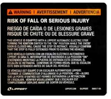
If the vehicle is driven with the step in the extended position, there is the possibility of causing major damage to both the step and the coach. Always be sure that the step is fully retracted before traveling. If the step is left extended and strikes an obstruction while the vehicle is moving, major damage to both the step and the vehicle could result.
