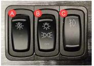
**(B) Headlamp Switch:** The headlamps can be turned on by the headlamp switch. In the first position, the switch will activate the marker, tail, identification, center, and clearance (ICC) lamps. The second position will activate the headlamps. While the headlamps are active, the turn signal lever can be pulled towards the driver to toggle between high and low beam operation. While vehicle ignition is on, an indicator in the instrument panel will be active whenever the high beam lamps are on.
