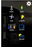
The KIB PANEL is a centralized "V-BUS" LCD interface to the following (if the coach is equipped):
