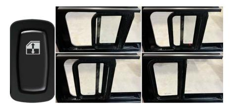
To close the window: Pressing up on the switch closes the window by sliding the window back and pushing the window out.
