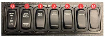
**(H) Generator Switch (Gen Start P. Heat):** The generator can be started from the rocker switch on the dash. Depending on the ambient temperatures, the generator may pre-heat prior to cranking. This pre-heat condition is noted by flashing the light on the generator start switch until the cycle is complete (up to 15 seconds). Once it has pre-heated sufficiently, the starter will engage and the engine will start.
