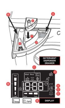
**Section A:** The duration of the available wash cycles and the remaining time of a running cycle appear in section A (Factors such as load size, modifiers, options selected, and water pressure may affect the time shown in the display. Tightly packed loads, unbalanced loads, or excessive suds may cause the washer to lengthen the cycle time as well); if the DELAYED START option has been set, the countdown to the start of the selected wash cycle will appear.
