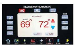
**Time Clock:** The HVAC controller is where the time of day is set and stored, there is a battery backup so even without power turned on the time of day is kept.
