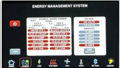
Once the EMS page has been opened, the Power button will allow the user to turn the Energy Management system on or off. When the EMS is off, it will allow the supply of power to all systems unregulated and may result in an overload of the incoming supply power and tripped shore power breaker(s). The power status information that is displayed on coaches with a factory-installed lithium package is supplied by the BMS, RVC transfer Switch and KIB and is not controllable from the KIB panel.
