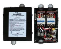
Automatic transfer switches are logic-controlled to convert under a given set of conditions. The transfer switches used in RVs are typically generator priority switches which connect to shore power under normal use. As soon as the transfer switch detects the presence of 120 Volt power on the generator input lines, it will switch over to the generator's inputs and drop the connection to shore power.
