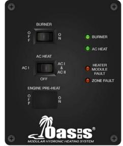
**Power LED (Green):** The power LED (green) turns ON when the power to the control board is ON. The LED flashes when the OASIS Heating Module is in Bypass mode.
