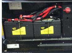
motorhome are installed by Newmar Corporation, but warranted by the battery manufacturer. These batteries are used to operate the 12 volt items that are not a direct part of the chassis.
