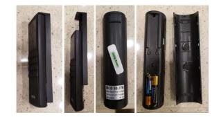
Replace the batteries. It is best to replace both batteries. If one defective battery is replaced, while leaving another weak or defective battery, lowered performance, or ultimately damaging the new or good batteries, may result. Reinstall the cover by placing it on the back of the remote and sliding it upward into place. To remount the remote, slide it back up into the wall mount.
