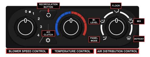
control dial will also control the overall temperature of the discharge air if the AC system is operating. Turn the knob to the right (red area) for warmer air, and to the left (blue area) for cooler air. Use of the temperature control will also moderate the discharge temperature when the cooling system is engaged.
