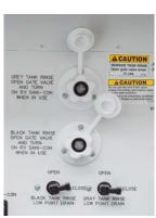
For coaches without low point drains for the tank rinse(s), the line to the vacuum breaker should automatically drain through the hose connection when the hose is disconnected, as this connection does not have a check valve.
