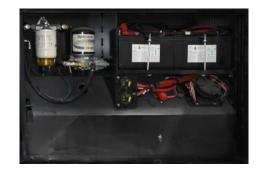
The inverter/charger will automatically charge the coach batteries when the unit is connected to a 120 volt outside power source and the batteries are connected via the charge bridge or BIM. The chassis batteries are isolated from the coach batteries. This prevents the chassis batteries from being drained by the interior 12 volt equipment, allowing ample voltage for engine ignition.
