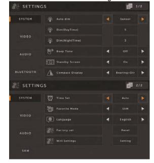
**Standby Screen:** Selecting ON, the Infotainment Center will display logo, date, time and temperature when the unit is powered on by pressing the power button (rotary button) while the vehicle remains on.
