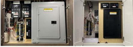
front overhead next to the 120 volt breaker panel, or the rear wardrobe. This panel contains fuses and breakers that are connected to the main appliances in the coach, from the refrigerator and television to the lights in the bedroom and slideouts. Some external components are fused in the house fuse panel. For example, the fuses for the water pump, water heater, security lights, and basement storage lights may be located in this panel.
