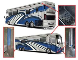
There are typically two drain pipes on the passenger side of the rear cap and one on each side of the front cap. The debris will come out the bottom of the coach if you are blowing it from the top, or the debris will come out the top of the coach if you are blowing it from the bottom.
