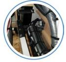
utilizing the coach water supply, are typically hard-plumbed within the slideout. To ensure flexibility, a braided hose connects the rigid plumbing from within the slideout to the rest of the plumbing in the coach. This hose easily moves with
