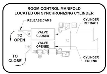
If the pump manifold is equipped with an auxiliary hand pump, you may be able to retract the room by opening only the room retract valve (as labeled by the wiring harness) and operating the hand pump, refer to the "Auxiliary Hand Pump Operation" page (in your HWH Operator's Manual) for instructions on the use of the hand pump and valves equipped with a release cam. If the room cannot be retracted with the hand pump, it will be necessary to use the lift bolts and room retract screws.
