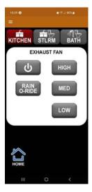
The fan operation screen provides buttons for On/Off and Rain Sensor Override, as well as the fan speed (High, Medium, or Low). A red button indicates the fan is currently in operation, which fan speed is selected, or the automatic rain-sensing technology is disabled (RAIN O-RIDE).
