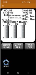
The water pump may be activated and deactivated via the KIB Monitor Panel, or, if equipped, via a momentary contact switch with LED indicator. The KIB switch panels communicate with a circuit board and touchscreen monitor on a dedicated V-BUS. The V-BUS receives on/off commands from the water pump button on the KIB display monitor or the water pump switch located in the water compartment.
