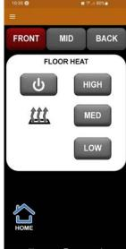
The different settings have specific on and off time intervals for heating. The heating indicator icon will illuminate when voltage is being sent to the heating element. For floor heat operation, 120 volts must be present from shore power or the generator.
