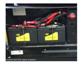
Depending on the coach, the batteries may be located in the front of the coach under the front cap or on a pull out tray in an outside compartment.
