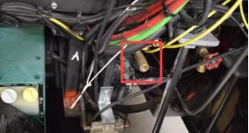
Coaches plumbed in this manner will have an additional Schrader valve port to allow pressurization during production.
