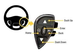
**Display:** The selectable display, located in the center of the screen, is controlled by the menu tabs to the left. Move up and down the tabs by using the up and down buttons on the steering wheel control. Each tab has a different display in the center.
