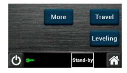
The ride height of the vehicle can be adjusted when traveling. Normal ride height is automatically selected by default. However, the ride height of the coach can be raised or lowered as needed. For example, high-ride may be selected to negotiate uneven terrain; likewise, low-ride may be selected to give additional clearance to the top of the vehicle.
