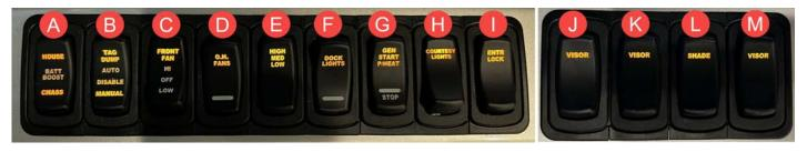
(A) Battery Boost Switch (Batt Boost): This switch allows the chassis battery to be boosted from the house battery bank or the house battery bank boosted from the chassis battery, allowing the solenoid to operate from either source that has power to engage the boost solenoid.
