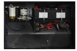
The chassis batteries are recharged by the vehicle's electrical system whenever the engine is running. With an added charge bridge solenoid or BIM, the vehicle's charging system will also charge house batteries if parameters are met.
