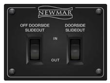
**Electric Bedroom Slideouts:** The operating switch for the bedroom slideout is usually located on the bedroom wall. If there is a full wall slideout on the driver side of the coach, the switch may be located on the wall that separates the bedroom from the living room.
