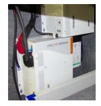
The inverter/charger can be controlled by a remote panel, from another system like SilverLeaf, or at the inverter itself. The remote panel is typically located in the front overhead compartment or above the entry door and is used to control the inverter and the battery charging functions. If a remote panel is connected to the inverter, then the remote panel takes priority.
