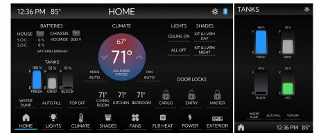
The water pump may be activated and deactivated via the ATC/KIB Monitor Panel. The KIB switch panels communicate with a circuit board and touchscreen monitor on a dedicated V-BUS. The V-BUS receives on/off commands from the water pump text on the KIB display monitor.
