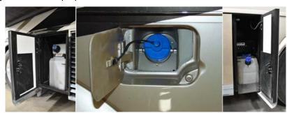
operation. For every 50 gallons of diesel fuel consumed, approximately 1 gallon of DEF will be consumed. Some vehicles are equipped with a remote DEF fill-port. If so equipped, the remote port is directly opposite the DEF tank on the other side of the vehicle, and has a blue cap over the fill-port. DEF parts, such as the fill cap or tank, are supplied by the chassis manufacturer and are not available via the Newmar Parts Department.
