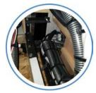
utilizing the coach water supply, are typically hard-plumbed within the slideout. To ensure flexibility, a braided hose connects the rigid plumbing from within the slideout to the rest of the plumbing in the coach. This hose easily moves with the slideout as it extends and retracts. The plumbing lines are normally tied to the flexible drain pipe and extend and retract smoothly as the slideout travels.
