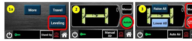
Press AUTO to initiate a leveling cycle. If the level controller will not go into Auto mode it is most likely because the vehicle's parking brake has not been applied, the vehicle is not in gear, or the ignition is off. Ensure the ignition is on, apply the parking brake, and put the transmission into neutral or park to allow the system to enter Auto mode.
