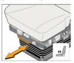
Enables the drivers to perform their job in a comfortable position. It provides a better view and easier accessibility of the dashboard. Pull the lever completely and move seat forwards/backwards. Once you have found your desired position, release the lever to lock the seat in place.
