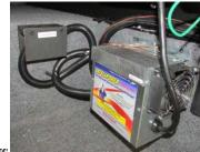
When replacing a converter, it is necessary to use the same size converter to ensure sufficient wining and preakers for the converter's input and output ratings.
