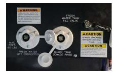
Before connecting to the coach, use a potable water source to purge any remaining air and stale water in the hose. Then, connect the hose from the potable water source to the coach. Turn on the supply valve at the water source, and open each of the faucets to remove any air pockets in the coach plumbing lines. Once the water flows freely, close the faucet(s).
