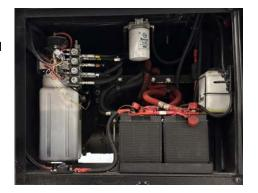
The inverter charger will automatically charge the coach batteries when the coach is connected to a 120 volt outside power source or if the generator is running. The chassis batteries are isolated from the coach batteries; however, when certain parameters are met, the BIRD, BIM, or charge bridge will activate and allow charge to the chassis battery. This prevents the chassis batteries from being drained by the interior 12 volt equipment and allows ample voltage for engine ignition.
