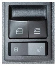
window will continue to roll down after the switch is released. Press the switch in the rearward position to raise the window.
