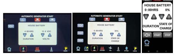
**Duration:** Time the AGS is to run the generator after a low battery demand occurs. Use "HR" & "MIN" buttons to set the amount of time the generator will run while charging the house or chassis batteries.
