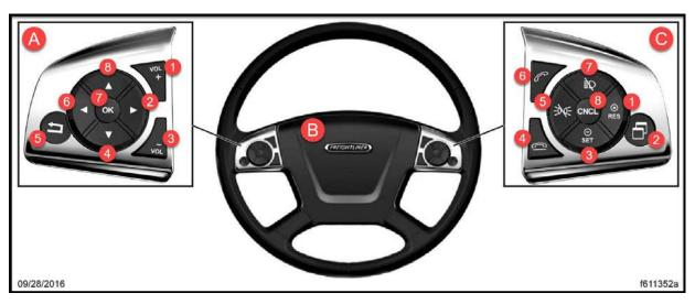
(A) Left-Hand Steering Wheel Switch Pod (Infotainment Controls)
