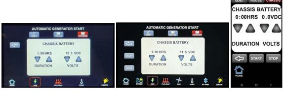
Example: If the house battery volts is "11.0 VDC" and the duration is "2:00 HRS," when the house battery voltage is less than 11.0 VDC, there will be a demand for the generator to start and run for 2:00 HRS. The chassis battery works the same way but with its own settings.
