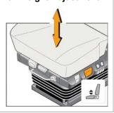
It supports the driver so that the pedals can be reached comfortably by the feet and passed through all the way without force.
