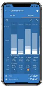
You can use the charge times to see if the PV array is properly sized for your requirements. A system that never reaches the float stage may need more panels. Or perhaps the load should be reduced?
