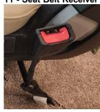
Seat belt assemblies are designed to secure persons in the vehicle to help reduce the chance of injury or the amount of injury resulting from accidents or sudden stops. Fasten the three-point seat belt by pushing the latch into the buckle. Listen for an audible click. Tug on the seat belt to make sure it is securely fastened.
