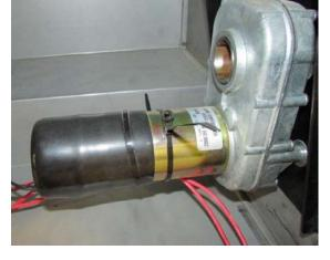
Depending on the year, model, and floorplan of the coach, the exact slideout motor(s) location may vary. Generally, they may be accessed from under the slideout in the compartment area. Some motors may also be located in the wheel well area under a cover.
