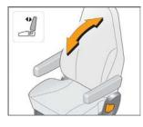
Enables the driver to stay in a comfortable position for a longer period of time by providing a custom inclination of the backrest. An upright position avoids postures with a high load on the back. Pull handle completely over the full adjustment stroke and adjust the backrest position by applying your back towards the backrest.
