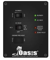
**Burner Switch (Primary Heat Source):** The burner switch on the remote panel controls the ON/OFF of the diesel burner. The Burner LED will turn on when the diesel burner has been activated, and will remain ON while the burner cycles on and off.
