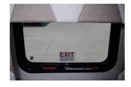
**In the event of an emergency, open the window:** Remove the screen by pulling out on the red handle. Push and release the lever from the locking hook. Rotate the lever 90 degrees, and push it through the slot in the window frame. Escape through the opening.
