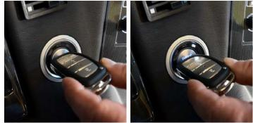
Press and hold the engine **START/STOP** button for more than one second with the Smart Key Fob to start the engine. The engine can start without depressing the brake pedal, but for your safety, always depress the brake pedal before starting the engine.
