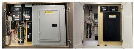
This panel contains fuses and breakers that are connected to the main appliances in the coach, from the refrigerator and television to the lights in the bedroom and slideouts. Some external components are fused in the house fuse panel. For example, the fuses for the water pump, water heater, security lights, and basement storage lights may be located in this panel.
