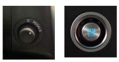
**(D) Keyless Ignition:** This vehicle ignition/starting system utilizes an electronic key fob in lieu of a mechanical key. The push button switch is used to activate accessory and ignition power and control the starting of the engine. To start the engine, depress the brake pedal and press the START/STOP ENGINE button with the transmission shifter in neutral (N). If the wait to start lamp is active, a second button press is required to start the engine.
