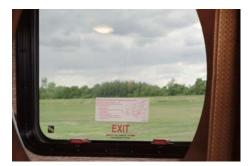
**To close the emergency exit double-latched window:** Pull the window shut while holding the window track with one hand. With the other hand, rotate the latch up until it connects with the track on the window. Press the front side down until it latches. Repeat the steps for the second latch.
