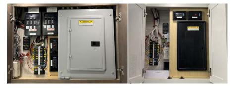
This panel contains fuses and breakers that are connected to the main appliances in the coach, from the refrigerator and television to the lights in the bedroom and slideouts. Some external components are fused in the house fuse panel. For example, the fuses for the water pump, water heater, security lights, and basement storage lights may be located in this panel.
