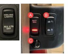
**(B) Visor Switch:** The passenger visor adjusts the passenger window screen up or down.
