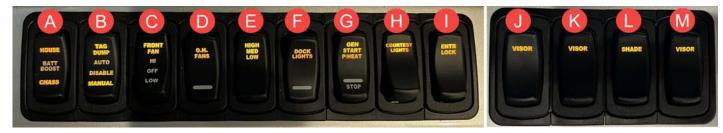
(A) Battery Boost Switch (Batt Boost): This switch allows the chassis battery to be boosted from the house battery bank or the house battery bank boosted from the chassis battery, allowing the solenoid to operate from either source that has power to engage the boost solenoid.
