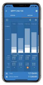
Clicking on any bar (day) in the graph will expand the information. It will show the time and percentage of the total charge time that the solar charger has spent in each Bulk, Absorption and Float charge stage.
