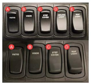
(E) Map Light Switch: The Map Light switch on the passenger console operates the light in the ceiling above the passenger seat by turning it on or off.
