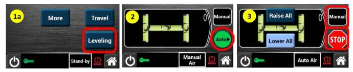
Press AUTO to initiate a leveling cycle. If the level controller will not go into Auto mode it is most likely because the vehicle's parking brake has not been applied, the vehicle is not in gear, or the ignition is off. Ensure the ignition is on, apply the parking brake, and put the transmission into neutral or park to allow the system to enter Auto mode.
