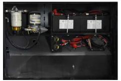
The Chassis Disconnect Switches are located in the rear passenger side compartment. There are two switches on a Spartan chassis, and when turned off, they will disconnect most of the chassis battery loads.
