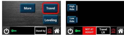
The leveling system can only be switched to travel mode causes the suspension to go to ride height.
