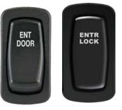
If the step is retracted, the step will extend anytime the door is opened. The step will retract anytime the door is closed unless the master door switch is off and the park brake is set.
