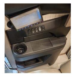
Switches: Ceiling Lights (All LTS Off), Battery Disconnect, Cargo Door Lock/Unlock, and Entrance Step Override
