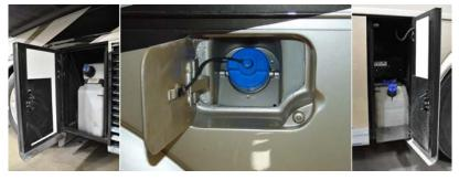
fuel consumption, dependent on vehicle operation. For every 50 gallons of diesel fuel consumed, approximately 1 gallon of DEF will be consumed.
