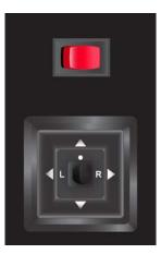
The adjustment control moves the top half of both mirrors. The bottom half of the mirror is convex and is adjusted manually.
