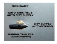
This condition may cause all faucets throughout the coach to provide warm or hot water from both the hot and cold positions. To prevent this condition, the Aqua View diverter valve should be left in the water flow position, except when trying to pre-heat the water to the shower faucet (just before taking a shower).
