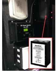
If there is no error message and the display instead reads "Delay Active" this means that the fault condition has cleared and that the switch is going through a 2.5 minute delay
