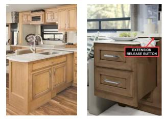
The cabinet "extension" is incorporated directly into the kitchen cabinetry, and glides out on drawer guides to provide additional counter space when needed. Coaches with particular floorplans are equipped with a counter extension and an electric latch release. To extend the counter:
