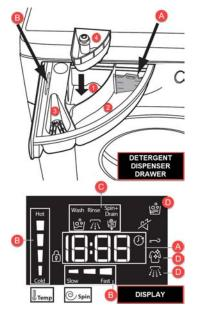
almost all sounds will be turned off. Only the sound signals and the alarms remain active, as well as the sound of the end of cycle. To activate/deactivate, press and hold the mute button.
