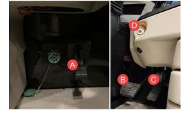
**(D) Keyless Ignition:** This vehicle ignition/starting system utilizes an electronic key FOB instead of a mechanical key. The push-button switch is used to activate accessory and ignition power and to control the starting of the engine.
