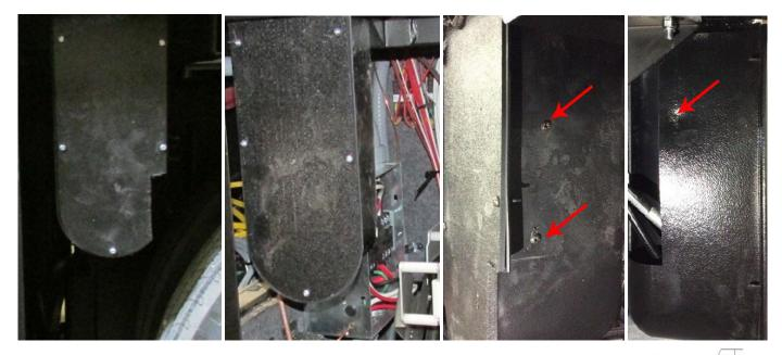
The lift bolt assembly may be mounted vertically or horizontally but will function the same way. Horizontallymounted lift bolts may not have a cover, depending on the location within the coach.
