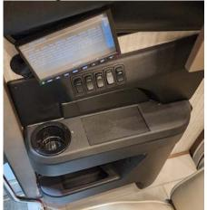
Switches: Ceiling Lights (All LTS Off), Battery Disconnect, Cargo Door Lock/Unlock, and Entrance Step Override
