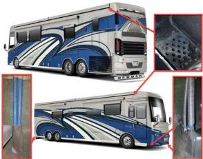
The debris will come out the bottom of the coach if you are blowing it from the top, or the debris will come out the top of the coach if you are blowing it from the bottom.
