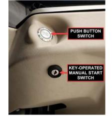
**Push to Start:** Pressing the engine start button will begin the process of detecting a FOB in range (J11P2 active). Our system will [check] the area of the driver. If the FOB is in range, it will respond with a single blink. If the FOB is authorized, our system will tell the motor that it may start.
