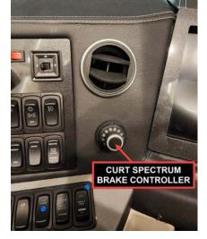
Pressing the control button switches between modes.
