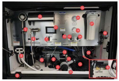
Water pressure levels above this level can damage the fresh water plumbing. If the water pressure ever surpasses 60 PSI, a pressure regulator must be installed to reduce the incoming pressure, or fill the fresh water tank and use the internal water pump to supply water to your coach.
