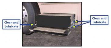
NOTE: Silicone lubricants and WD-40® are not recommended for use. They have a tendency to evaporate and dry the mating surfaces which leave them vulnerable to the elements.
