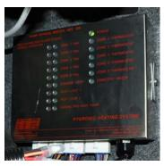
When the "series" jumper is not in place, the zone control board uses Heating Loop 1 to supply coolant to Zones 1 and 2, and uses Heating Loop 2 to supply coolant to Zones 3, 4, and 5. Zones 1 and 2 are calling for heat, the zone control board will activate the Heat Loop 1 pump. When Zones 3, 4, and 5 are calling for heat, the zone control board will activate the Heat Loop 2 pump.
