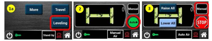
Press AUTO to initiate a leveling cycle. If the level controller will not go into Auto mode it is most likely because the vehicle's parking brake has not been applied, the vehicle is not in gear, or the ignition is off. Ensure the ignition is on, apply the parking brake, and put the transmission into neutral or park to allow the system to enter Auto mode.
