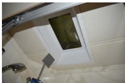
Periodic cleaning using a mild detergent or cleaner specifically designed for plastics (such as Novus No. 1) is necessary; cleaning frequency may depend on the surrounding conditions while driving, parking, or storing the coach.
