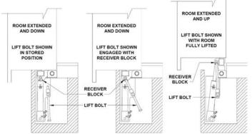
receiver block. Continue to turn the bolt(s) until the room is completely lifted. When there are multiple lift bolts, alternate evenly between all lift bolts, turning each bolt two or three complete turns each time. Turning one lift bolt without alternating may cause the room to bind.
