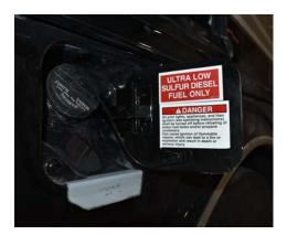
All pilot lights, appliances, and their igniters (see operating instructions) shall be turned off before refueling of motor fuel tanks and/or propane containers. Can cause ignition of flammable vapors, which can lead to a fire or explosion and result in death or serious injury.
