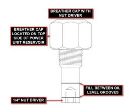
The oil level should be within one inch of the top of the reservoir. Most breather caps have a dipstick. Fluid level should be between the bottom of the dipstick and the center mark.
