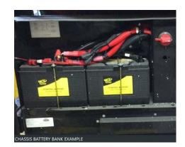
These batteries are used to operate the 12 volt items that are not a direct part of the chassis.
