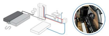
utilizing the coach water supply, are typically hard-plumbed within the slideout. To ensure flexibility, a braided hose connects the rigid plumbing from within the slideout to the rest of the plumbing in the coach. This hose easily moves with
