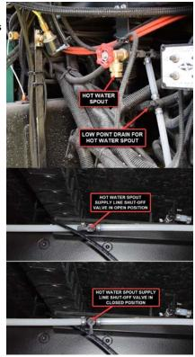
Note: If you plan to drive in cold temperatures without the rest of the coach winterized, simply close the supply line shutoff valve located in a basement compartment and open the low point drain near the hot water spout. This will shut off the water supply to the hot water spout and prevent it from freezing in cold temperatures.
