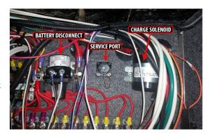
When a 12 Volt load or component is not working, both 12 Volt power (+) and 12 Volt ground (-) are needed for the load to complete the 12 Volt circuit.
