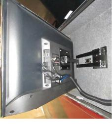
It is important to make sure the TV is securely locked into position prior to closing the compartment door. Failure to do so can result in damage to the television case and screen.
