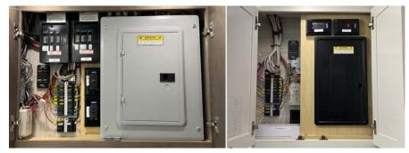
This panel contains fuses and breakers that are connected to the main appliances in the coach, from the refrigerator and television to the lights in the bedroom and slideouts.
