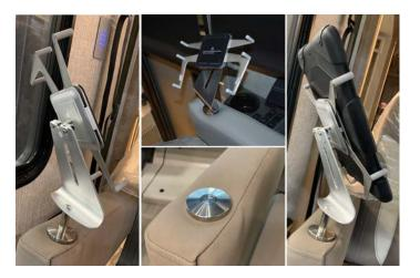
Adjust the clamps' angle and place your device on the proper location of the cradle, then secure your device with six clamps (adjust the size by moving the arms, legs, and feet of the holder to fit the size of the desired device). Rotate the cradle clockwise or counterclockwise to adjust the angle. Turn the cradle downward or upward to adjust the angle.
