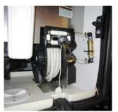
Note: The house battery disconnect must be turned on for the power hose reel to be operated.
