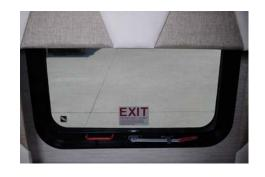
**To close the vent:** Unclip the red handle from the latch by lifting slightly while pushing outward. Once the latch releases, pull the arm in until the window is closed. Rotate the arm 90 degrees until it latches into the closed position.
