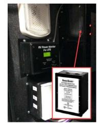
If no display is available, check the level of the input voltage to ensure it is within the proper operating limits. Also check that the ATS is correctly connected to chassis ground and that the neutral conductor is correctly connected to ground at the power pedestal. Wait 2.5 minutes to check if the fault condition was temporary and has cleared. If so, the contactor will pull in at the end of the 2.5 minute period.
