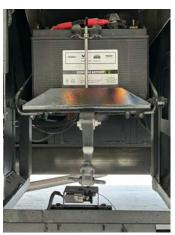
The chassis batteries are isolated from the coach batteries; however, when certain parameters are met, the BIRD, BIM, or charge bridge will activate and allow charge to the chassis battery. This prevents the chassis batteries from being drained by the interior 12 volt equipment and allows ample voltage for engine ignition.
