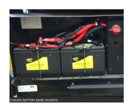
motorhome are installed by Newmar Corporation, but warranted by the battery manufacturer. These batteries are used to operate the 12 volt items that are not a direct part of the chassis.
