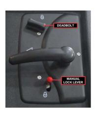
To lock the door without using the deadbolt, press and hold the number one key on the keyless entry touchpad (if equipped). Flip the red lever before shutting the door, or use the key fob (if equipped).
