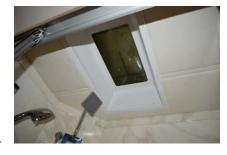
Newmar recommends using Surebond SB-140 butyl sealant around the skylight. Periodic cleaning using a mild detergent or cleaner specifically designed for plastics (such as Novus No. 1) is necessary; cleaning frequency may depend on the surrounding conditions while driving, parking, or storing the coach.
