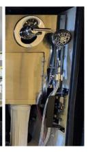
Each tank has its own control valve, and both tanks drain through the sewer drain hose. The waste water system catches and contains the used water and divert the waste water through the traps and drain lines to the grey or black holding tank(s). It is then stored until the tanks are emptied using a sanitary drain or dump station.
