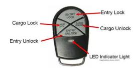
While the engine is running, only the entry unlock function of the e-FOB remains activated — other functions are deactivated.
