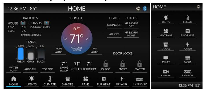
The Home screen on the 2026 High End User Interface displays an overview of the tank capacities and other water-related functions, voltage monitoring, main lighting and shade controls, as well as access to the main icons at the bottom of the screen: Lights, Climate (HVAC), Shades, Fans, Floor Heat, Power, and Exterior.
