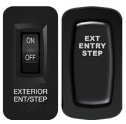
The only time the step will stay extended is if the door is open or if the door is closed with the park brake on and the master step switch off.
