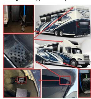
The drains can be blown out using compressed air (approximately 60 PSI) from the drain pipes found under the front and rear caps of the main cabin area. There are typically two drain pipes on the passenger side of the rear cap and one on each side of the front cap.
