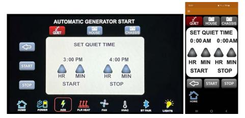
Note: The time of day is set in the HVAC section and must be set for operation. For example, RV parks have posted times when generators are not to run, and the user simply enters those times and enables the "QUIET" button on the status page. During this time, the generator will not run.
