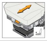
Enables the driver to adapt the length of the cushion to the length of their thighs. It helps to keep the feet and lower legs from "falling asleep" and provides a safer and more fatigue-proof posture. Adjust the cushion so that 3 fingers fit in between the cushion's front edge and behind the operator's knee. Pull the lever and move the seat cushion forward/backward. Release the lever to lock the seat.
