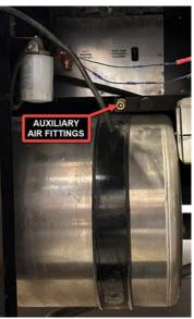
This auxiliary input fitting can be used to inflate the air system from an outside source such as a shop air compressor or tow truck). The auxiliary output fitting can be used to inflate floats, bike tires, or car tires.
