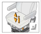
Protects the spine of the driver, as the damper absorbs the vertical shocks and vibrations. By adjusting the damper, the suspension characteristics of the seat can be optimally adapted to every roadway and every driver.
