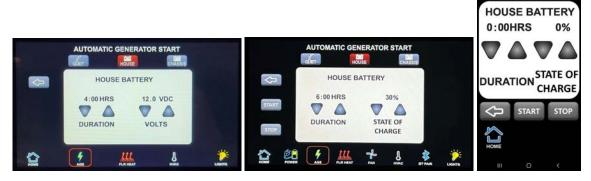
**Duration:** Time the AGS is to run the generator after a low battery demand occurs. Use "HR" & "MIN" buttons to set the amount of time the generator will run while charging the house or chassis batteries.
