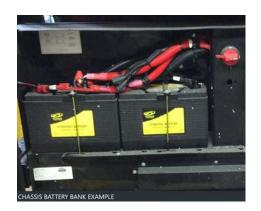
These batteries are used to operate the 12 volt items that are not a direct part of the chassis. Depending on the coach, the batteries may be located in the front of the coach under the front cap or on a pull out tray in an outside compartment.
