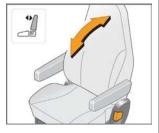
Enables the driver to stay in a comfortable position for a longer period of time by providing a custom inclination of the backrest. An upright position avoids postures with a high load on the back. Pull handle completely over the full adjustment stroke and adjust the backrest position by applying your back towards the backrest.
