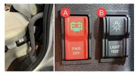
(A) Smart Battery Shut-Off Switch (Battery Disconnect)
