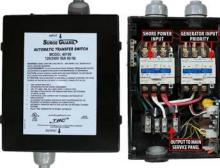
As soon as the transfer switch detects the presence of 120 Volt power on the generator input lines, it will switch over to the generator's inputs and drop the connection to shore power.
