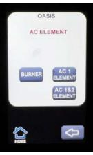
AC 1 or AC 1 & 2 Element Buttons (Secondary Heat Source): The AC 1 Element and AC 1 & 2 Element buttons control activation of a single 120 VAC immersion element or both 120 VAC immersion elements jointly. The AC Element buttons will change color to indicate when the element(s) have been activated.
