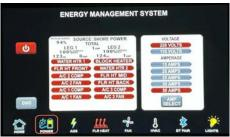
Once the EMS page has been opened, the Power button will allow the user to turn the Energy Management system on or off. When the EMS is off, it will allow the supply of power to all systems unregulated and may result in an overload of the incoming supply power and tripped shore power breaker(s).
