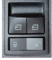
Hold the switch down in the forward position for approximately one second to activate the express function; the window will continue to roll down after the switch is released. Press the switch in the rearward position to raise the window.
