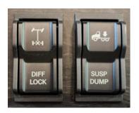
A status screen showing engaged locks is found in the vehicle operations menus on the driver display. Each differential lock is controlled by a switch on the dash.
