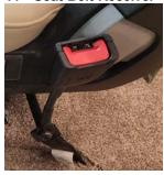
Seat belt assemblies are designed to secure persons in the vehicle to help reduce the chance of injury or the amount of injury resulting from accidents or sudden stops. Fasten the three-point seat belt by pushing the latch into the buckle. Listen for an audible click. Tug on the seat belt to make sure it is securely fastened.
