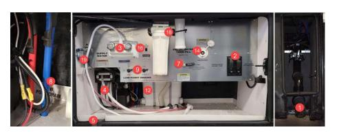
**Water Pressure Requirements:** Ease of operation was the key element in the design of the water compartment and plumbing systems. The fresh water system in your coach is designed to operate at a maximum of 60 PSI. Water pressure levels above this level can damage the fresh water plumbing. If the water pressure ever surpasses 60 PSI, a pressure regulator must be installed to reduce the incoming pressure, or fill the fresh water tank and use the internal water pump to supply water to your coach.
