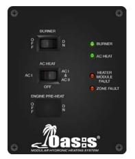
**Burner Switch (Primary Heat Source):** The burner switch on the remote panel controls the ON/OFF of the diesel burner. The Burner LED will turn on when the diesel burner has been activated, and will remain ON while the burner cycles on and off.
