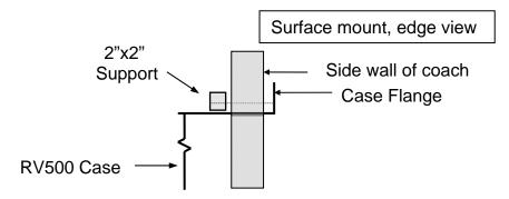
Attach a 3/4"thick 2 x 2" wide wood spacer to the bottom of the cut out. This will center the flange of the RV-500 vertically in the opening. This applies if you are installing the RV-500 in either the flush or surface mount configuration.
