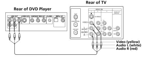
For better picture quality, use S VIDEO instead of the yellow video cable. S VIDEO does not provide sound; you still must connect the audio cables.
