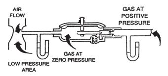
The greater the airflow through the carburetor venturi, the lower the pressure at the venturi throat. The lower the pressure at the venturi throat, the greater the diaphragm movement, and the greater the movement of the regulator valve. The more the regulator valve opens, the greater the gas flow that is proportional to airflow through the generator.
