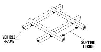
The generator can be installed so that it sits on top of the horizontal support tubing if the vehicle design permits. Another method is to suspend the generator below the horizontal support tubing by means of suitable, structurally sound metal framework. The following general rules apply:
