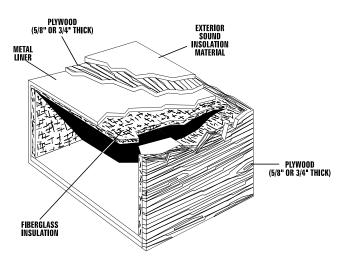
• Line the compartment door interior (except for air openings) with suitable, fireproof sound insulation (such as 1-inch (25 mm) thick fiberglass with a 2-pound density).
