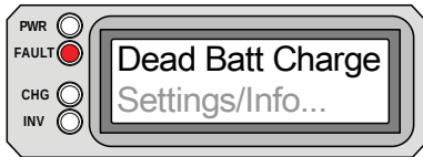
Figure 5-18, Dead Battery Charge Fault
