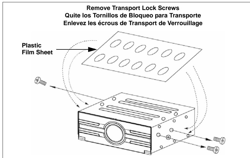
**CAUTION!** After removing the three transport lock screws, place three pieces of the small plastic film (supplied) over the three screw holes to prevent water entry.
