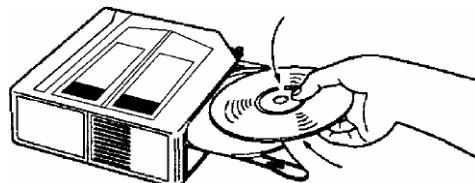
3. Push the tray back into the magazine. Load discs into the remaining 9 trays in a similar manner.
