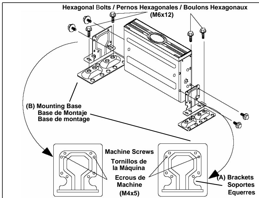
4. Determine the mounting location and mount the unit.
