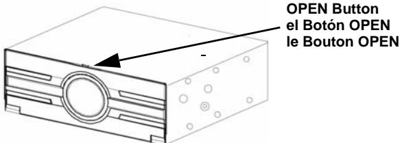
2. Making sure the top of the magazine is facing upward, gently insert it into the unit until it clicks into place.
