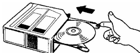
**NOTE:** This unit is not designed to play 3" (8cm) CD-Single discs. Inserting a 3" disc into the magazine, either with or without a 3" disc adaptor, can damage the changer and the disc. Such damage will not be covered by the Warranty on this product.
