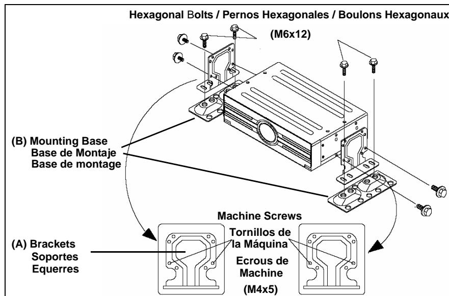
4. Determine the mounting location and mount the unit.
