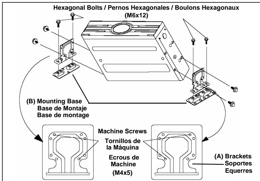
4. Determine the mounting location and mount the unit.
