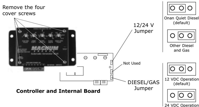
**Figure 1 - AGS Controller Configuration
