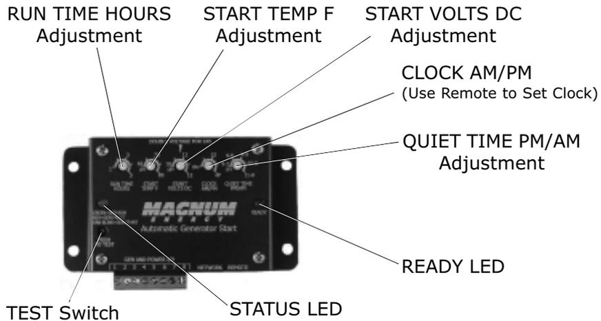
**Figure 5 - AGS Controller Adjustments (Run Time Hours, Start Temp F, and Start Volts DC)**
