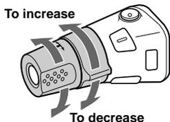
If you need to mount the rotary commander on the right hand side of the steering column, you can reverse the operative direction.
