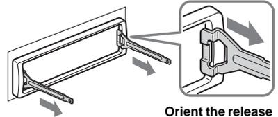
Orient the release key correctly.
