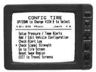
Using the up  $\Delta$  or down  $\nabla$  keys move arrow to Check Signal Strength.
