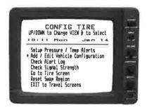
Using the up  $\triangle$  or down  $\nabla$  keys move arrow to Check Alert Log.
