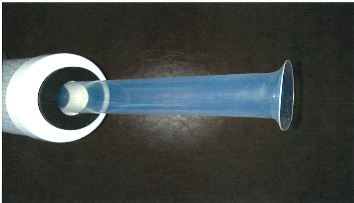
Figure 5 filter #2 end with Teflon sleeve protruding this should be inserted in filter before black gasket is installed see attached sheets
