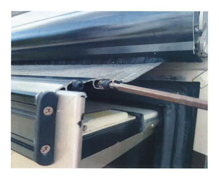
• Align awning fabric tube into frame.
