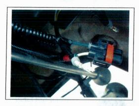
13. Insert the colored wire of the auxiliary harness into its corresponding connector for each light.
