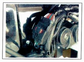
1. Locate where the headlight harness mates with the chassis harness behind the front hood door.
