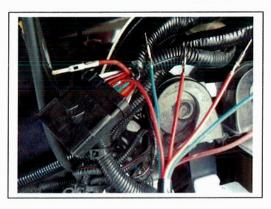
8. Insert the terminal of each wire of the auxiliary harness into its corresponding pin location of the harness connector.
