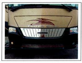
19. Locate and remove the Left Headlight 15 Amp CB from the fuse panel. Turn on the lo-beam headlights and fog lights. Verify that only the Right lights are on. Repeat for Hi-Beam lights. Turn off headlight and fog lights. Replace CB in the fuse panel.
