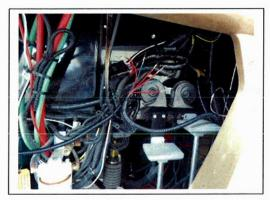
Loosely install and route the auxiliary harness along the headlight harness.
