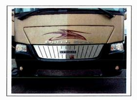
18. Turn on the lo-beam headlights and fog lights. Verify that both Left and Right lights are on. Turn off headlights and fog lights.
