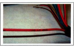
7. Identify each of the six wires with terminals at the center of the auxiliary harness. Each wire is stamped with the circuit name as shown above in Step #4.
