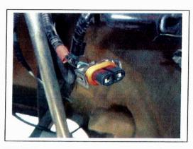
10. Remove the harness connectors that plug into the Lo-Beam, Hi-Beam and Fog lights.
