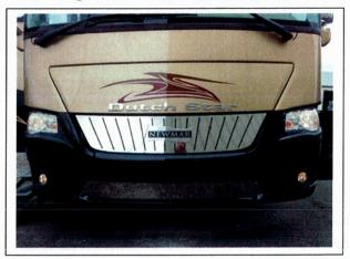
Turn on the lo-beam headlights and fog lights. Verify that both Left and Right lights are on. Turn off headlights and fog lights.
