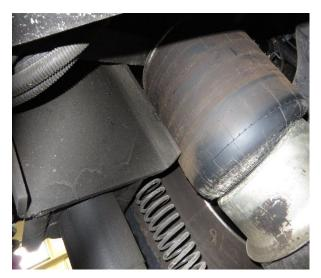
If less than 3/4 of inch is showing than the radius portion of the "U" channel will need removed.
