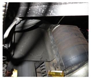
• Starting below the chassis railing, cut the channel radius off down to the bottom edge of bracket.
