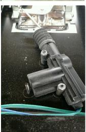
Then install the new actuator, and tighten down with the two Nylock nuts.
