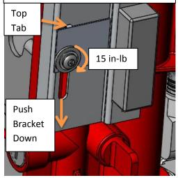
2) Place stop key onto bracket with tabs inside the slot. Finger tighten screw through lock washer and washer.
