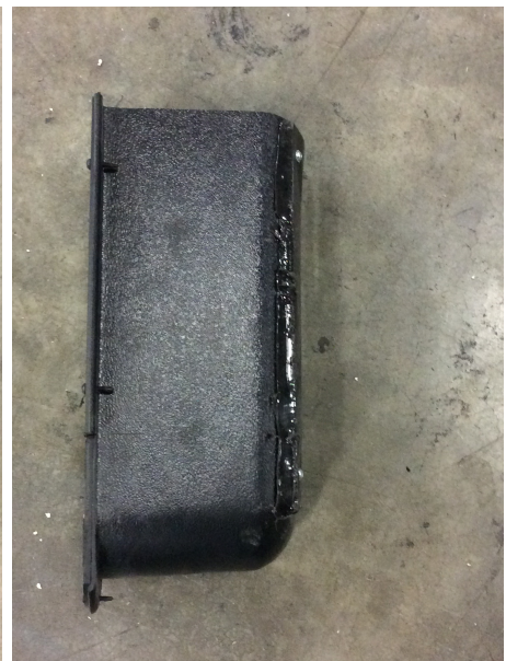
After Flap Installation and Sealant Applied
