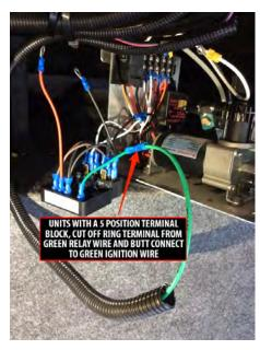
On coaches equipped with a 5-position terminal block, cut the ring terminal off the new relay. Then strip the insulation and connect it to the green wire using a blue butt connector.
