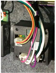
Locate the pink wire with a green stripe (ignition wire) connecting to the slideout modules nearby.
