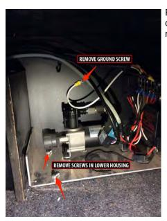
Remove the ground wire and mounting screws. Pull the power door opener control system to the edge of compartment ledge to access and install the new module.
