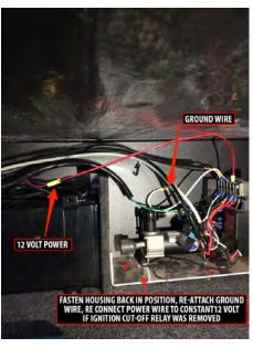
Place the control assembly back into position. Then refasten it with screws, and reattach the ground wire.
