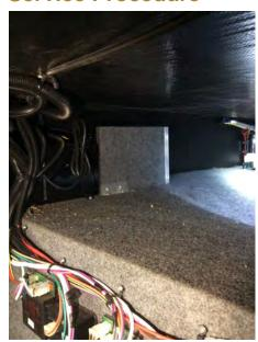
Remove the cover around the door control. The control assembly is usually located in one of the storage compartments near the handicap door and in front of the rear axle on the passenger side.
