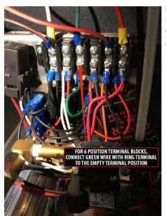
On coaches equipped with a 6-position terminal block, hook up the green wire to the open space in the terminal block.
