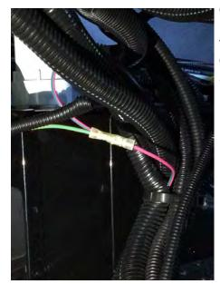
Cut the pink and green wire, and strip the insulation from both ends.
