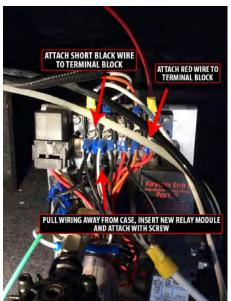
Move the wiring around, and install the new relay delay assembly against the metal housing under the terminal block.
