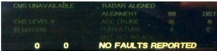
19. Start the coach, and press the service brake with your foot. Release the park brake, and press the diagnostic button twice on the glass dash controller.
