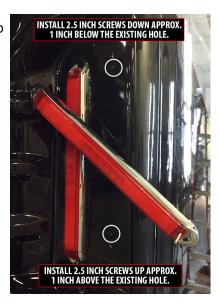
3. Reinstall the tail light using stainless 2-1/2" self-tapping pan head screws.
