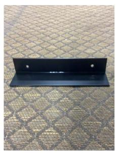
1. Prep the angle pieces to be mounted. Drill one 3/16" hole in each end of the narrower side of the angle. Each hole should be centered and approximately one inch from the end of the angle piece (as shown).
