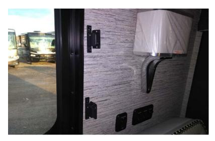
9. Put the valance in place, and secure them to the other side of the Friction Catches using 8x½" screws (part #136072).
