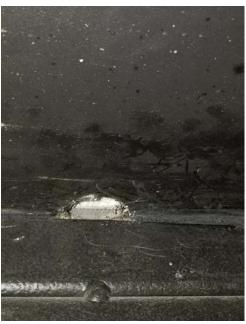
5. From the wheel well, use spray foam to fill the cavity in the floor.
