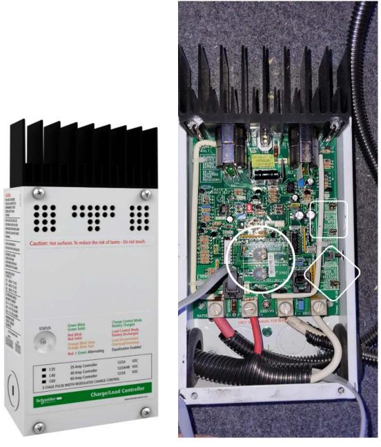
Remove the four screws on the front cover. Check and adjust the setting as described on the recall.
