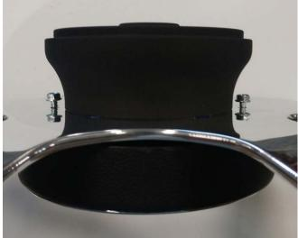
3. Using a 4 mm Allen wrench or socket, remove the five cap screws that were exposed after the center cover was removed. Add Loctite 243 to each bolt. It is recommended to remove one at a time, and then thread each bolt by hand.
