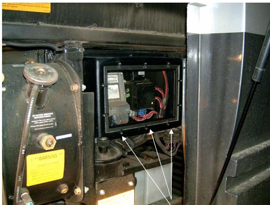
Picture 4 Clear plastic cover on box (note retaining clips).
