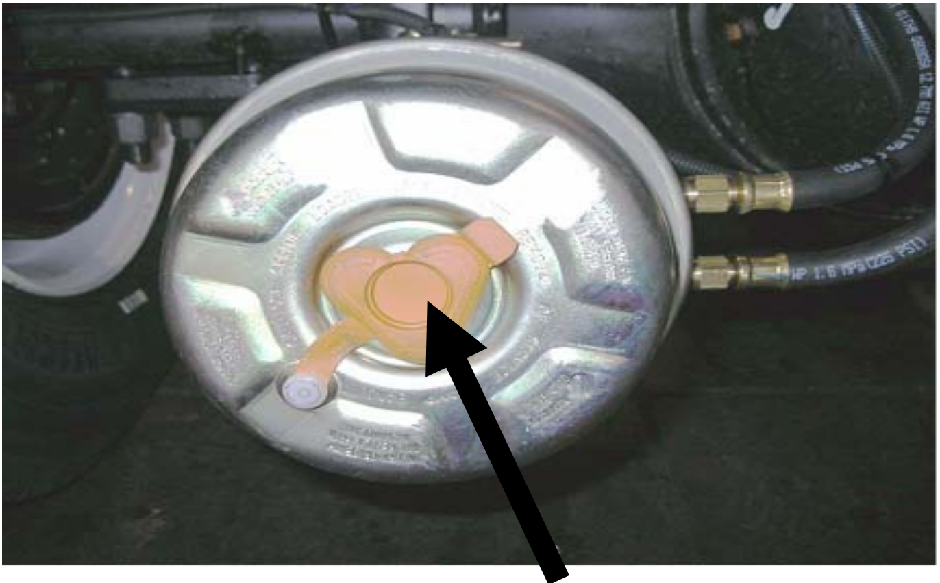
Properly installed Dust Plug in Haldex Brake Chamber
