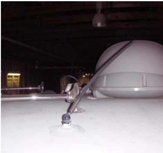
Figure 2 - Upon replacement of the 12" black rubber AM/FM antenna mast, please make sure that the tip of the mast is pointed to the rear of the coach and is in approximately a 60 degree angle.
