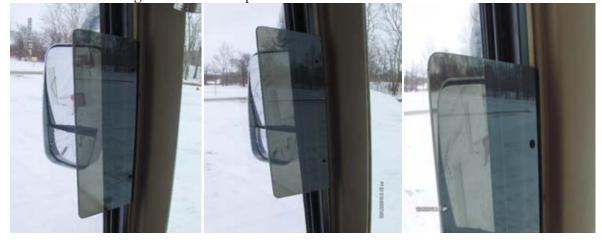
2) Remove the protective film from both sides of the shield, place the Plexiglas shield back on the window trim in the proper location and use ½" self tapping screws to secure the shield in place.
