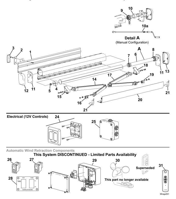
Electronic components shown are not used for the Direct Response system.
