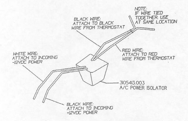
This isolator will filter out most AC volts that may cause erratic air conditioner operation.
