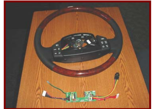
FIG. 2-1 CIRCUIT BOARD SHOWN REMOVED FROM HOUSING
