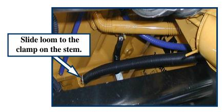
DIPSTICK TUBE WITH LOOM FIG. 3-2
