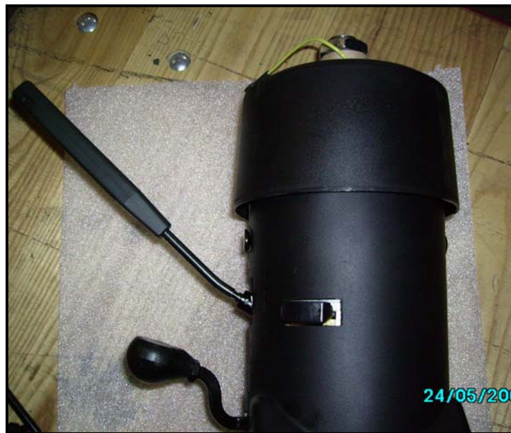
COLUMN SHOWN WITH NEW TURN SIGNAL STALK
