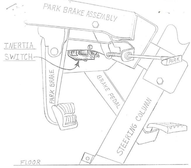
VIEW: LOOKING THRU DRIVERS DOOR AT L.H. SIDE OF STEERING COLUMN. PARK BRAKE IN THE "SET" POSITION
