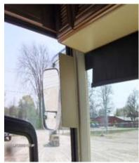
1) Place the Plexiglas shield onto the driver's side window trim to determine proper location for installation. Mark 2-3 locations on the forward edge of the shield for the screws to be installed. Pre-drill the holes for the mounting screws with the protective film still attached.
